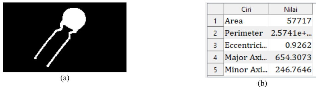
Figure 5. (a) Morphological Operation Image, (b) Feature Extraction Results
