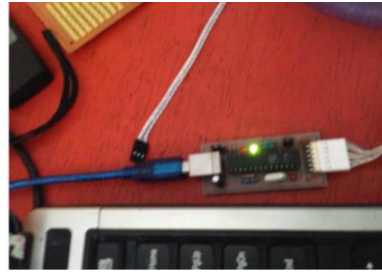
Figure 10. Downloader transfers data to IC with Raspberry Pi
