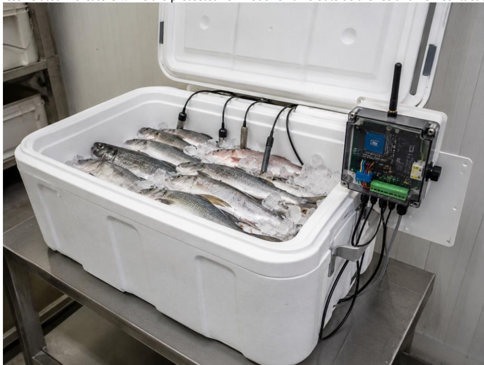
Figure 6. Illustrative visualization of the monitored fish-storage box and sensor placement
